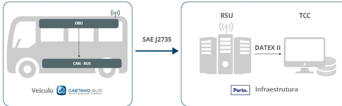
Unidirectional communications between the OBU in the BUS, the RSU and the Oporto TCC:
