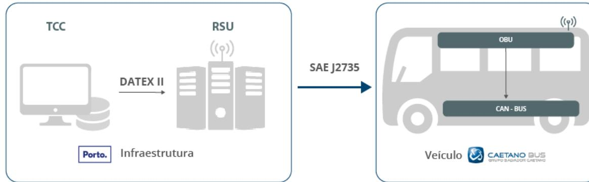
Unidirectional communication between Oporto (TCC), the RSU and the OBU in the BUS:
