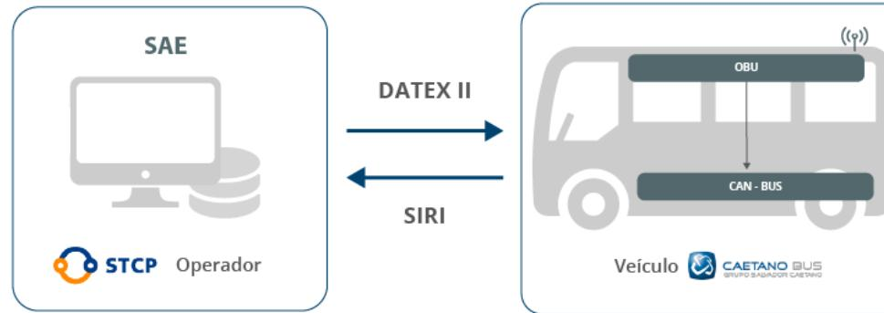
Bidirectional communication between STCP (SAE) and the OBU in the BUS:
